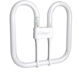
New 2D<sup>™</sup> Watt-Miser<sup>™</sup> lamps are energy saving compact fluorescent tubes formed into a "2D" shape. All types are available with a 4pin cap which permits use with conventional or electronic (high frequency) control gear, dimming and emergency lighting circuits. The 16-28W types are also available with 2pin cap which contains a starter switch and an EMC (RIS) capacitor.
